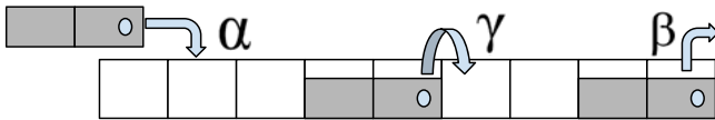
Fig. 1. The codon-based lattice model for mRNA translation, where the ribosome covers two codons on the mRNA. The entry and exit of the ribosome are assumed to be instantaneous. \alpha , \beta , and \gamma are initiation, termination, and elongation rate constants, respectively.
