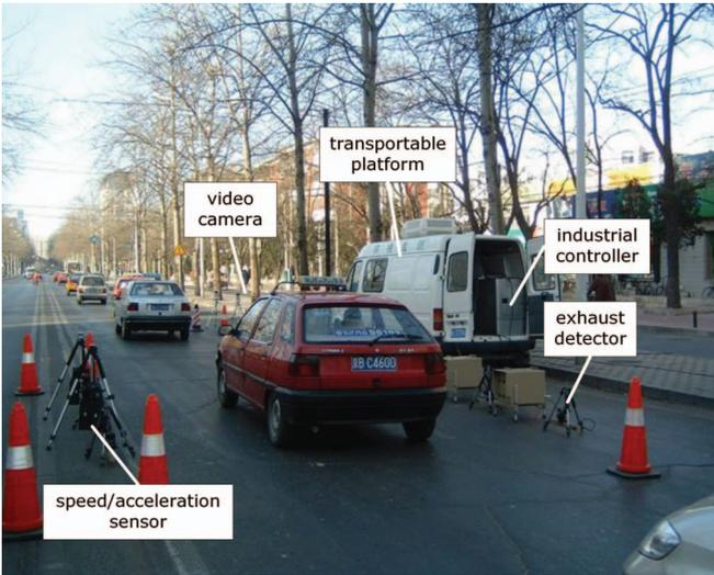
Fig. 1: Illustrating the transportable vehicle emissions remote sensing system.
