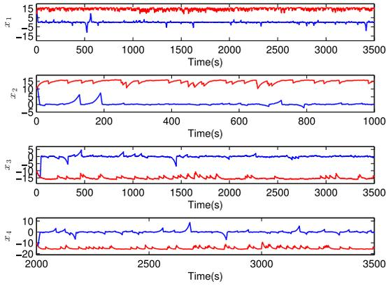
Fig. 6. State responses with packet-based compensation. The blue line is obtained by PBMPIC and the red line is obtained without active compensation.
