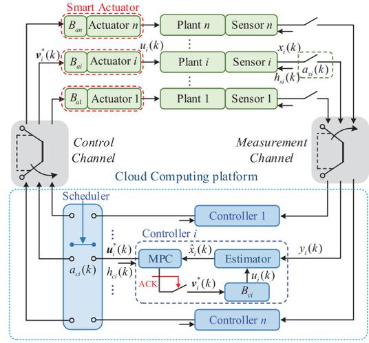
Fig. 2. Dual scheduling PBMPC framework for WCCS, where  $B_{ai}$  and  $B_{ci}$  are the buffers for actuator  $i$  and controller  $i$ , respectively.  $u_i^*$  is the output control signal of PBMPC while  $v_i^*$  is the received one by the actuator.
