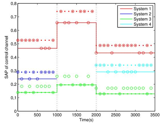
Fig. 5. Comparison of the SAPs obtained by i.i.d. scheduling (solid lines), threshold strategy with fixed priority (solid points), and threshold strategy with random priority (empty circles).
