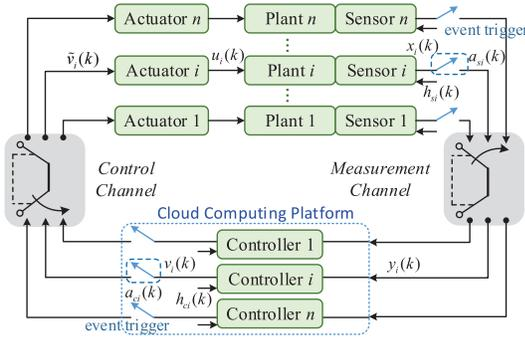
Fig. 1. Illustrating the system structure of wireless cloud control systems, where the controllers of all systems are implemented at the cloud computing platform.  $h_{si}/h_{ci}$  (time  $k$  is omitted and subscript  $i$  means system  $i$ ) is the channel gain of the measurement/control channel;  $x_i/y_i$  is the input/output signal of the measurement channel;  $v_i/\tilde{v}_i$  is the input/output signal of the control channel; and  $u_i$  is the control input.
