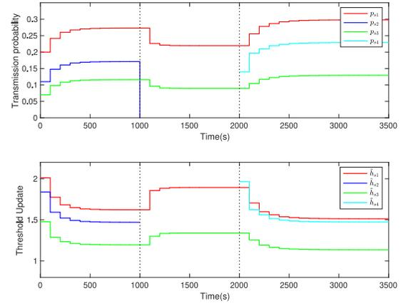
Fig. 4. Update of access probability  $p_{si}(k)$  for each sensor computed by the best-response dynamic (17) or better-response dynamic (18) with  $\beta = 0$ , and the update of the realted threshold level  $\tilde{h}_{si}(k)$  of the access strategy.
