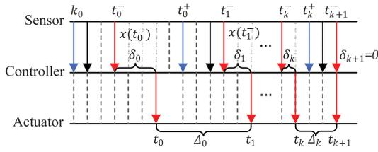
Fig. 3. Example of state/control packet transmissions among sensor, controller, and actuator with possible packet losses.
