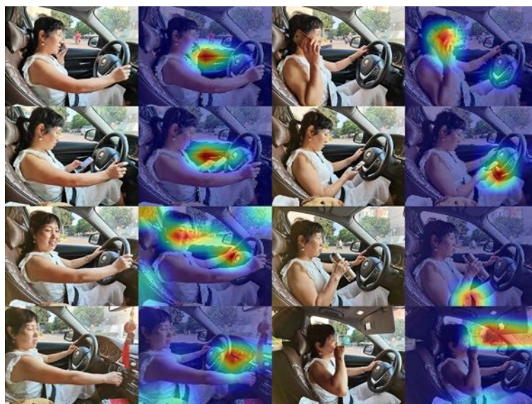
图 4-12 ResNet50 算法在“ZJUT- Districted-Driver-Detection”数据集上的热力图 Figure 4-12. Heat map of ResNet50 algorithm on "ZJUT- Districted-Driver-Detection" dataset
