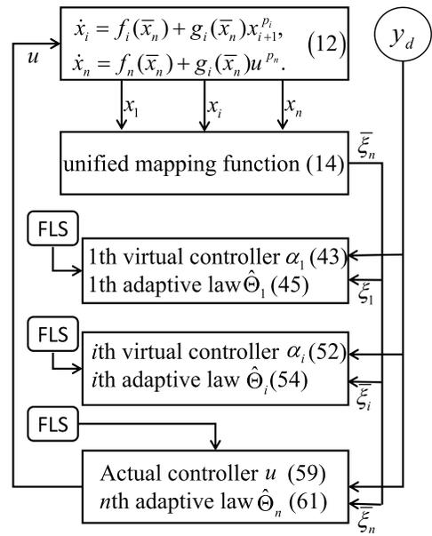
Fig. 1. Flow chart of control algorithm.
