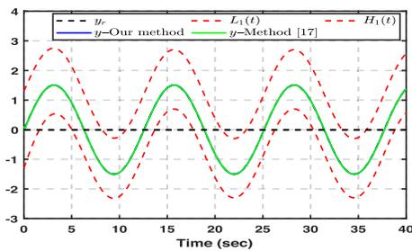
Fig. 5. Tracking curves of our method and the method in [19].
