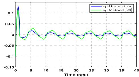
Fig. 3. Tracking error curves under our method and the method in [31].
