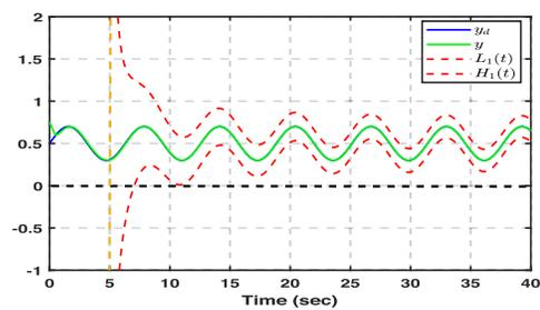
Fig. 8. Desired signal  $y_d$ , system output  $y$  and its boundary functions.
